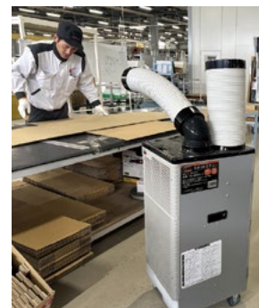
Preventing heatstroke at the Gotemba Plant: Spot coolers
