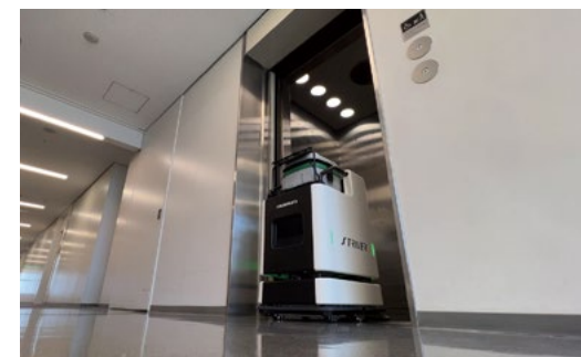
Linking robots with elevators
