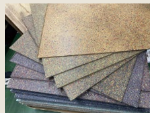
One-of-a-kind PANECO® boards, reprocessed from scraps into material
